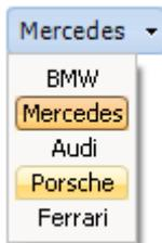
It is equally possible to create a tool selector with custom drawn tool items. This is done through the OnDrawTool event that is triggered for every item. Where for a normal selectors, the size of a button in the panel is derived from the ToolImages imagelist width & height, for a custom drawn selector, this is set with OwnerDrawWidth & OwnerDrawHeight. Here is a sample of a custom tool selector with full code:
